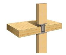
CLT floor slabs with glulam columns and steel connectors
